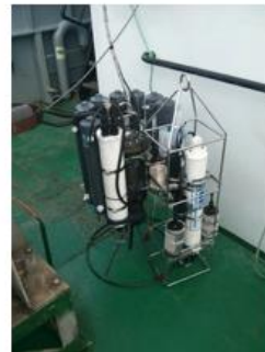
Optode sensors mounted on CTD frame ready for deployment (image courtesy E. Fritzsche)
